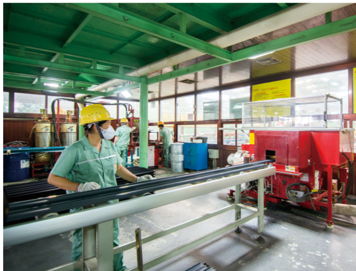
隔热穿条车间 Thermal Break Plant of Bar-insertion
